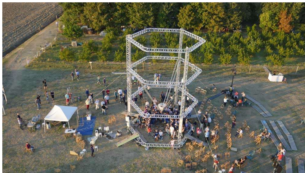
Figure S1. The BigDelta 3D printer made by WASP [source WASP].
